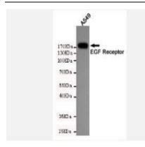
Western blot detection of EGFR in A549 cell lysates using EGFR mouse mAb(dilution 1:2000). Predicted band size:134 Kda. Observed band size:175 KDa.
